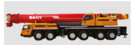
SAC3000 Max. lifting capacity: 300 t, Main boom: 7 sections, Extension boom: 15.4-80 m, Chassis: 12x8x12
