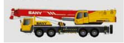
STC300B Max. lifting capacity: 30 t, Main boom: 4 sections, Extension boom: 10.65-33.5 m, Chassis: 8x4x4
