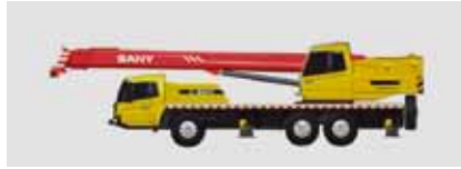
STC250C-5 Max. lifting capacity: 25 t, Main boom: 5 sections, Extension boom: 10.5-39.5 m, Chassis: 6x4x2
