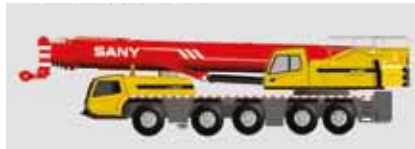
SAC2200 Max. lifting capacity: 220 t, Main boom: 6 sections, Extension boom: 13.5-62 m, Chassis: 10x8x10
